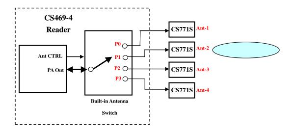
The CS469-4 switch is at time slot-2 at this moment. The port-1 is turned on. So only Ant-2 is active for transmitting the power at this moment.
