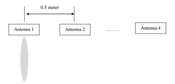
Energy coming out of 1 antenna (note that CS469-4 is switched on in time one by one so that at any 1 moment in time ONLY 1 antenna is turned on)
