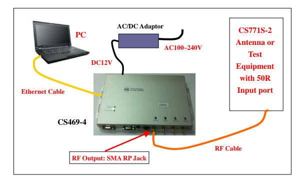
Figure 4-5 12V power adaptor mode Setup
