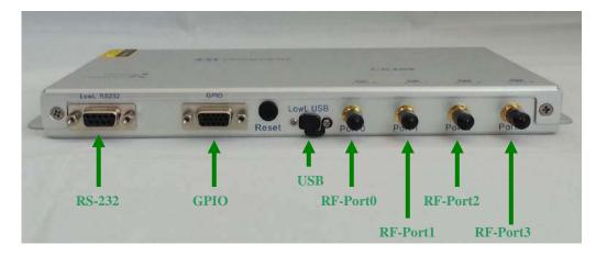
Figure 4-2 CS469 Reader Side View
