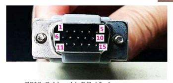
GPIO Cable with DE-15 plug
