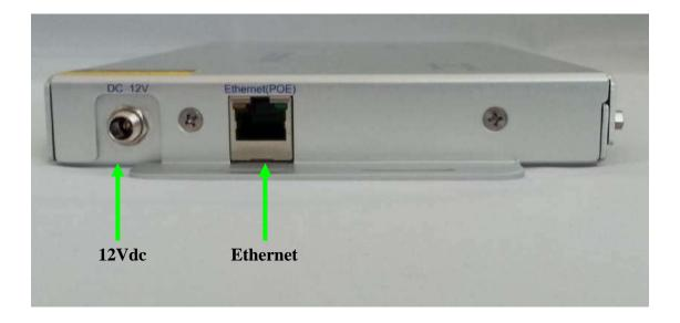
Figure 4-3 CS469 Reader Side View
