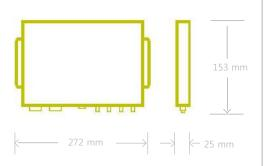
CS469 4-Port Reader is an Ethernet POE connected UHF EPC C1 G2 RFID reader with long read range (12 meters with Dogbone tags from Smartrac) and high read rate (300 tags per second). The high performance level, combined with affordable price, makes the CS469 the best total cost solution in the industry. With the same API as CS203 and CS468 - CSL Unified API, the application development time and cost are reduced, resulting in a faster time to market.
