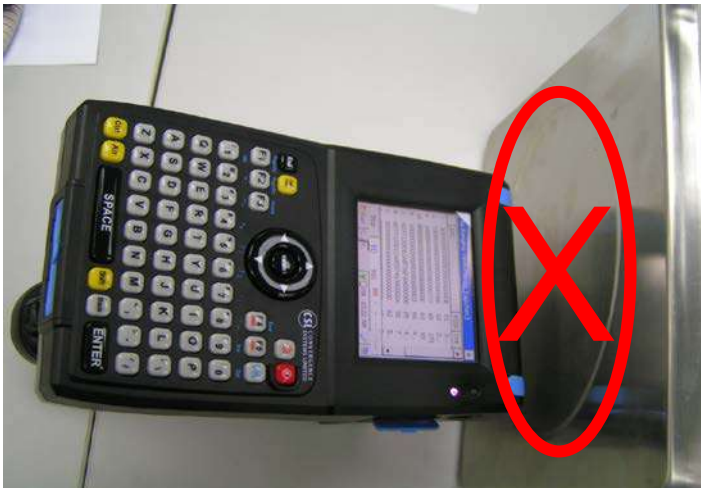
Reader antenna too close to metal
