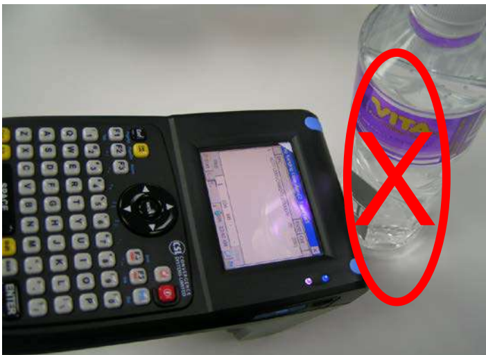
Reader antenna too close to the tag
