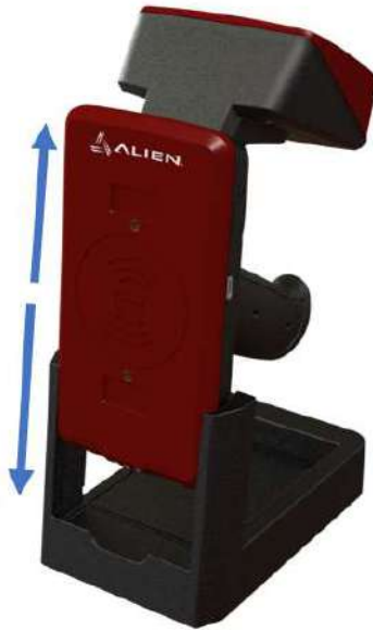
Figure 5: Charging of the Alien ALR-S350 via the ALX-540 cradle
